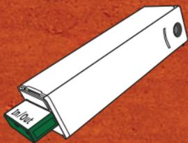
Insert the battery at the bottom of the device.
