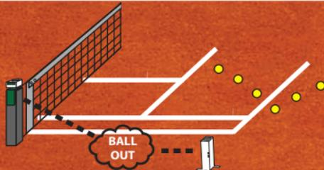
For close calls, data is sent over-the-air from the line device to the net device.
