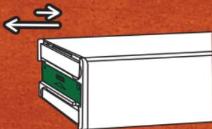
To remove the battery, push it inwards. The clip will eject it.
