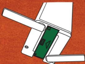
For better stability, rotate the pads below the device.
